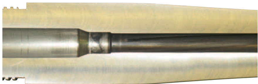
An eroded barrel will affect precision
